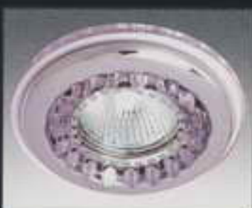
Item: 2125 Size: 100×55mm Hole Size: 80mm Halogen MR16
